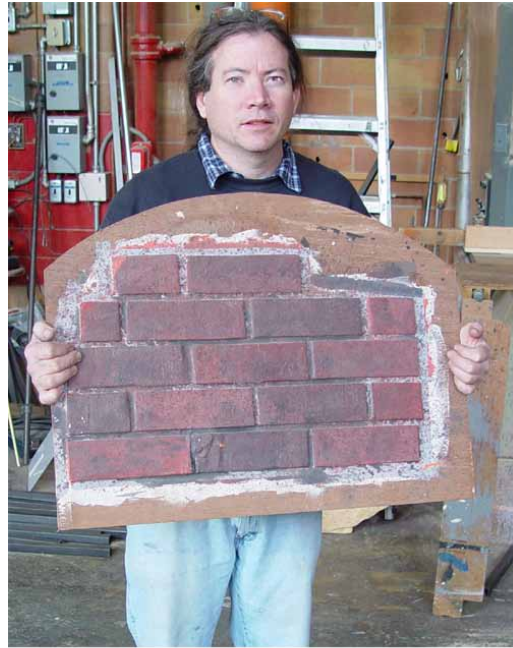
AUTHOR HOLDS A SAMPLE BOARD OF BRICK TEXTURE MADE BY USING FOAM RUBBER
